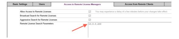
After a few minutes the network key should be visible at <a href="http://localhost:1947/devices.html">http://localhost:1947/devices.html</a>
